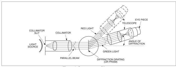
Figure 1 Spectrometer Diagram
