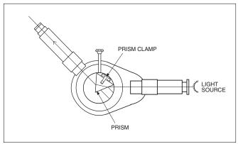
Figure 10 Mounting the Prism
