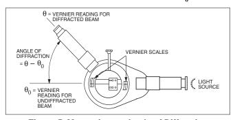
Figure 5 Measuring an Angle of Diffraction
