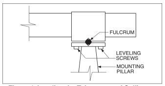
Figure 4 Leveling the Telescope and Collimator
