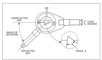
Figure 9 Angle of Deviation
