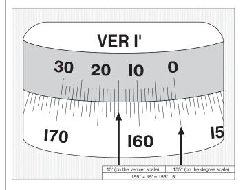
Figure 6 Reading the Vernier Scales
